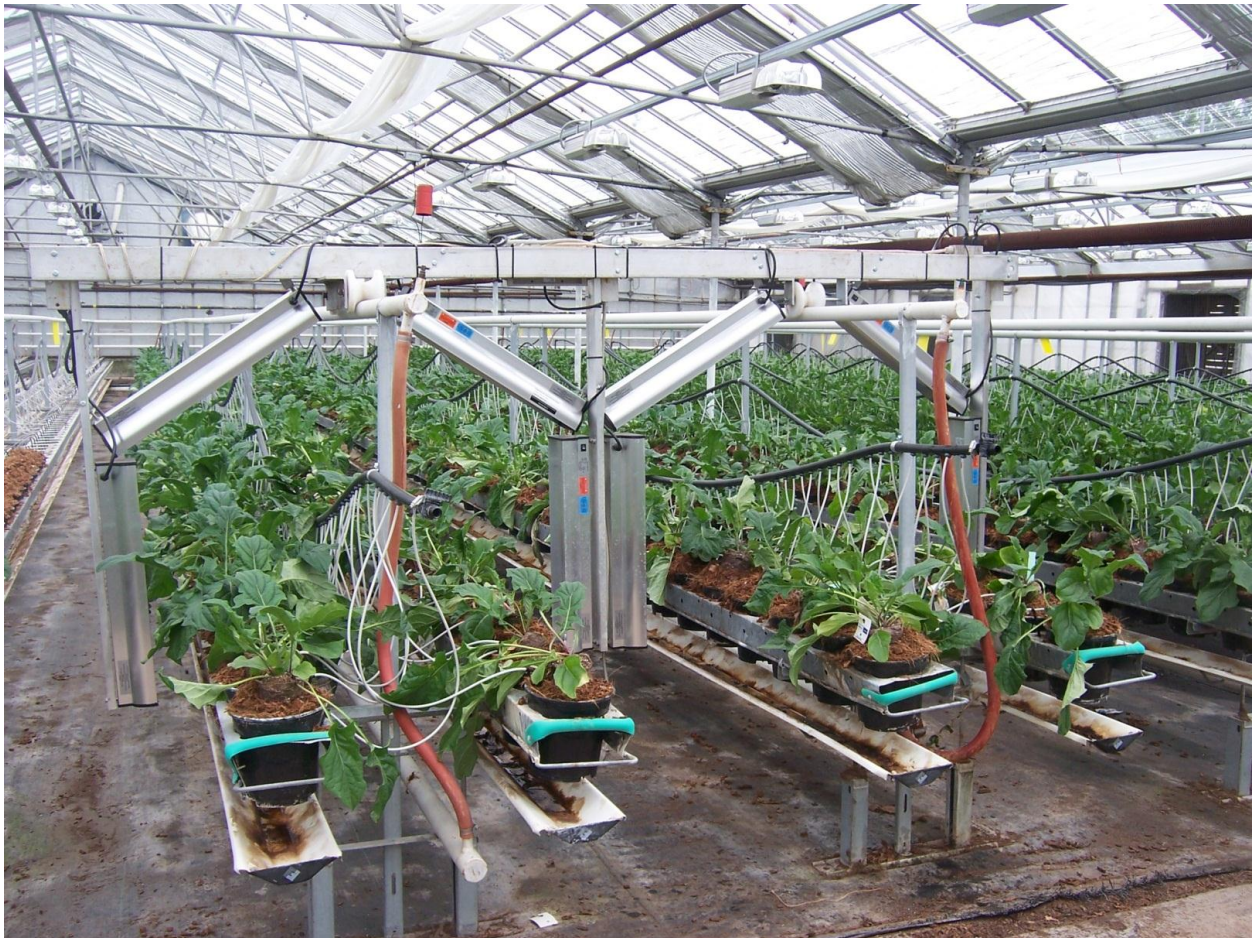
Figure 1. Light arrangement for trial to provide exposure to top and along sides of crop canopy. Light modules added to picking carts in specific arrangement to provide optimal coverage of plants while dosing with ultraviolet C. Trial will include gerbera varieties Nuance, Bayadere and Soul Sister.
